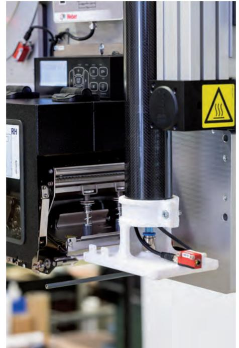
For use in particularly harsh environmental conditions (also with heating), IPC in the protective enclosure, Bluhmware for system control and interlinking, Legitronic® label printing software, label presence check, scanner (1-D/2-D), vision systems, sensors, RFID gates, product sensors, product height recognition, variable dispensing stroke sensing, tripod in different versions (stationary and spindle-adjustable)
